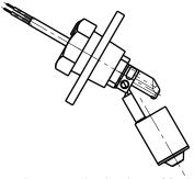
Make sure it is installed in horizontal position
