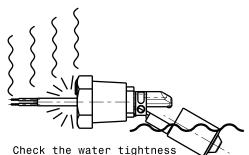
between the float assembly and the cable assembly
