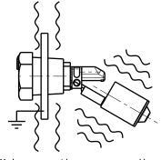
Make sure ther are no vibrations in the installation area A specific request is otherwise necessary
