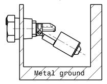
Do not install in the vicinity of a magnetic metal ground Risk of modification or disturbance in the detection
